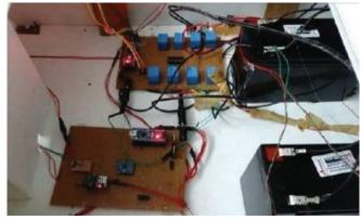
Fig. 5. Internal Circuit of IoT Based Robot
