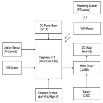
Fig. 1. Block diagram of proposed System
